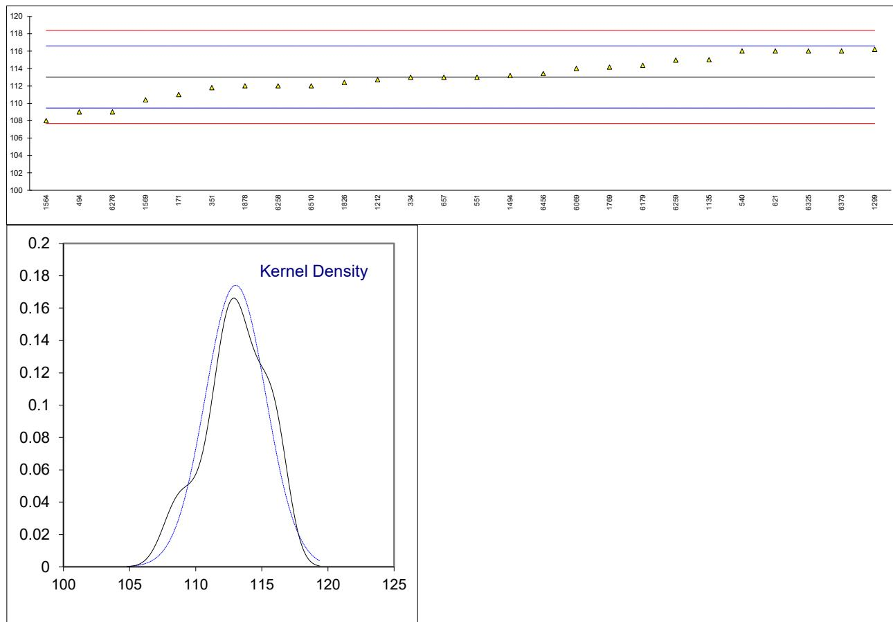
Determination of Kinematic Viscosity at 40 °C on sample #23060; results in mm<sup>2</sup>/s
