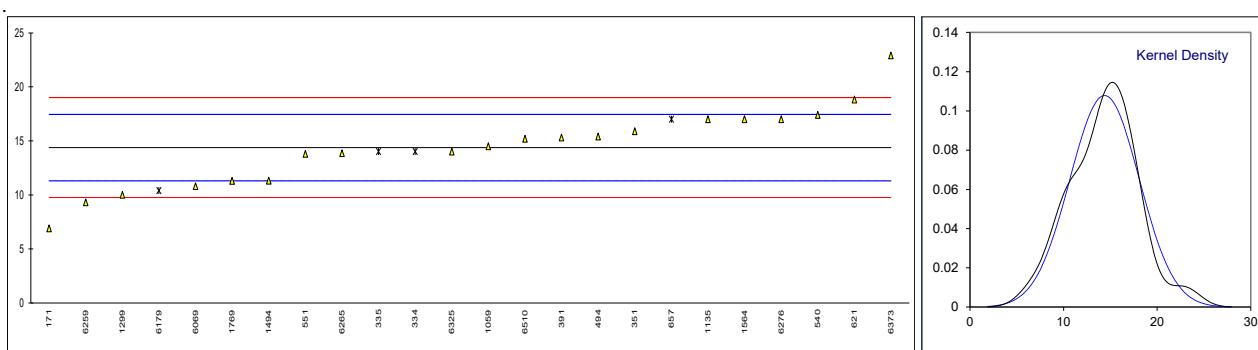
Determination of Filter Blocking Potential by Cold Soak Filterability Test (CSFT) on sample #23063; results in s
